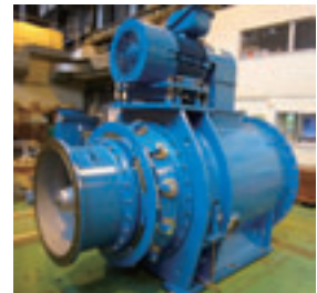
Hydroelectric power generation equipment for sewage treatment plants (Hydro-eKIDS™ type L)
