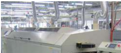
Reflow furnace in the PWB production line
